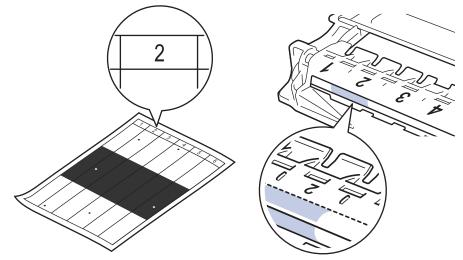
11. Turn the edge of the drum unit towards you while looking at the drum surface to find the mark.
