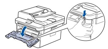
3. Remove the toner cartridge and drum unit assembly from the machine.
