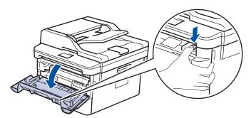
7. Remove the toner cartridge and drum unit assembly from the machine.
