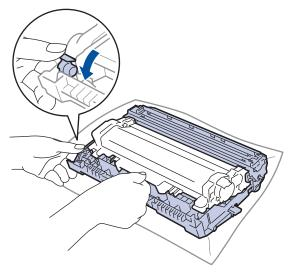
9. Turn the drum unit as shown in the illustration. Make sure that the drum unit gear is on the left side.
