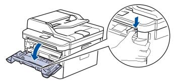
3. Remove the toner cartridge and drum unit assembly.
