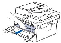
3. Clean the corona wire inside the drum unit by gently sliding the green tab from left to right and right to left several times.
