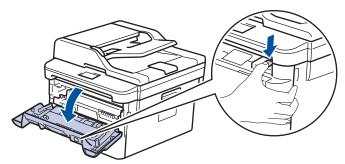
3. Remove the toner cartridge and drum unit assembly from the machine.
