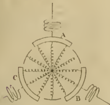
FIG. 5.—DIAGRAM OF OPEN-CIRCUIT ARMATURE WITH SEVERAL BRANCHES IN PARALLEL UNDER WIDE BRUSH BELONGING TO EACH PHASE.
