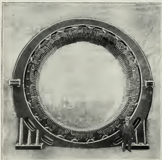
FIG. 10.—STATOR OF 11,000-K.V.A. THREE-PHASE ALTERNATOR.
