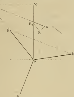
FIG. 8.—CONSTRUCTION FOR FINDING THE VOLTAGE REQUIRED TO BE GENERATED BY ADVANCER.
