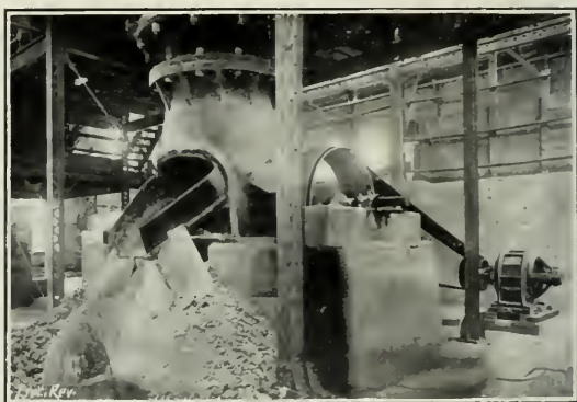
FIG. 6.—A 150-H.P. ROCK CRUSHER DRIVE.
