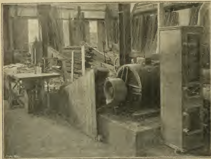
LEA VALLEY MILLS: 30-H.P. MOTORS AND "CONSPED" CONTROLLERS DRIVING LINE SHAFTS.
