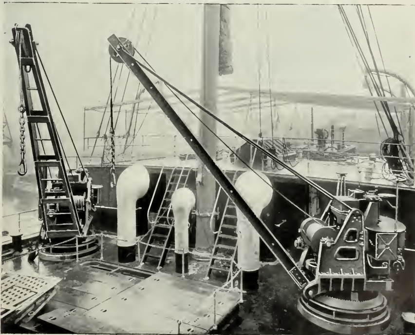
ELECTRIC CRANES ON THE AFTER DECK, SS. "FAUVETTE."
