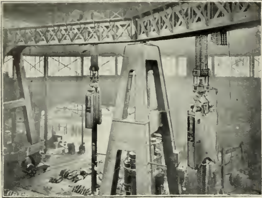
FIG. 5.—TWIN GANTRY CRANE OF 120 TONS' CAPACITY.
