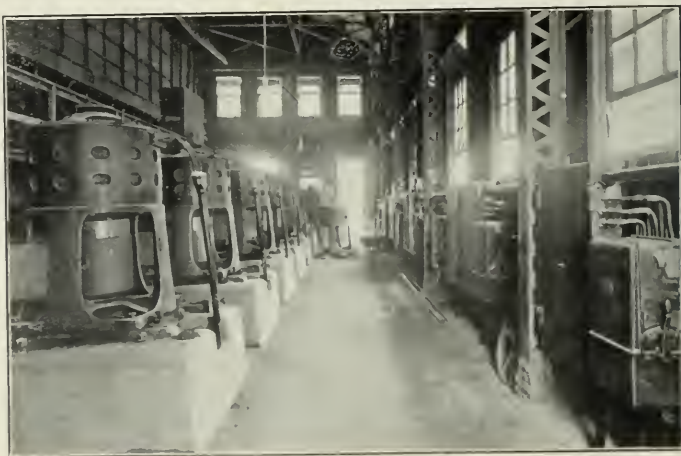
FIG. 7.—GROUP OF TEN 75-H.P. VERTICAL MOTORS DRIVING FULLER MILLS
