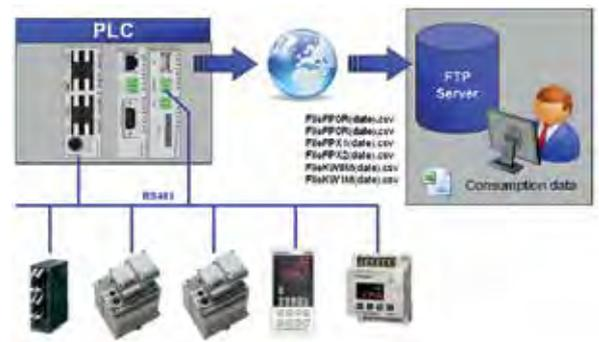
Panasonic presents the **FP Web-Server 2 (FPWEB2)** as a hub of the Smart Machine: a small device that adds advanced functionality to any machine.
