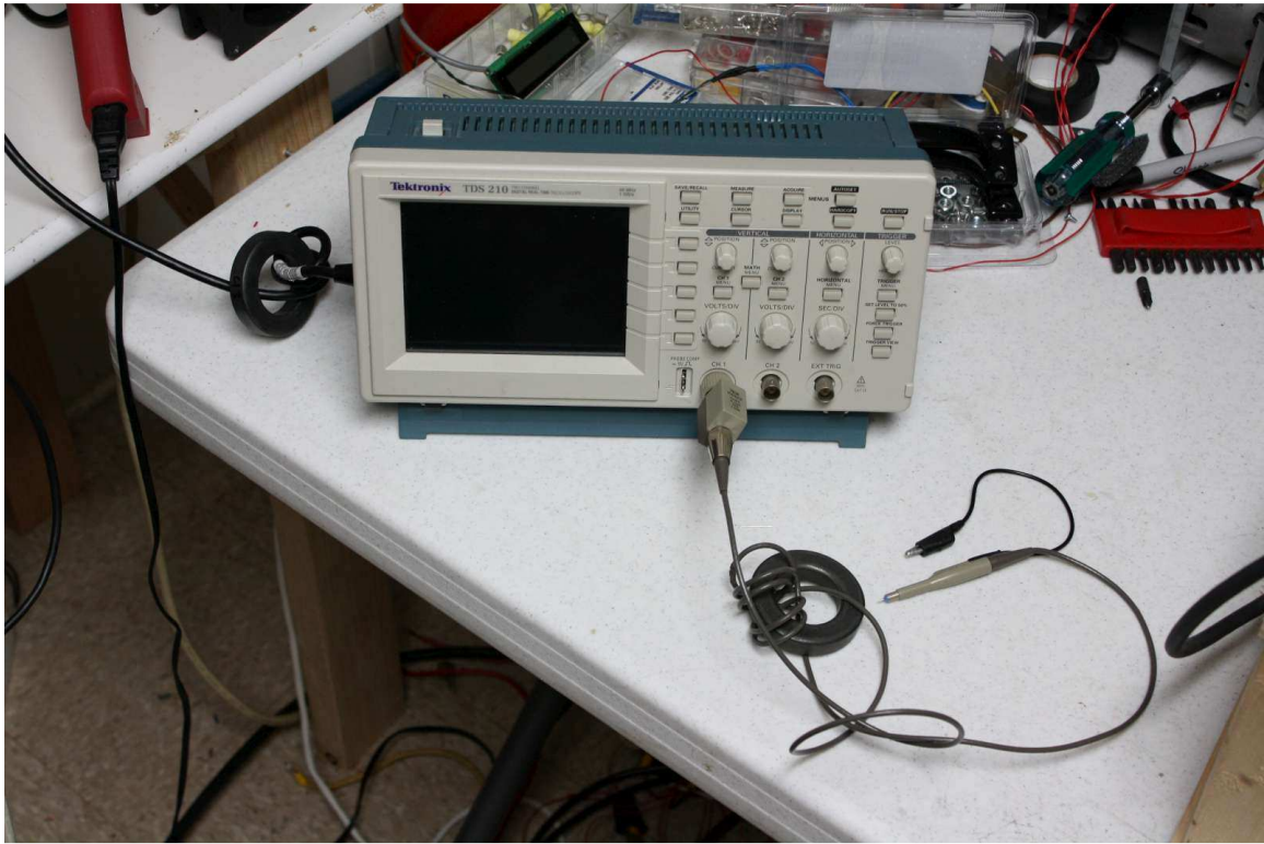
TDS210 with Common-Mode filters
