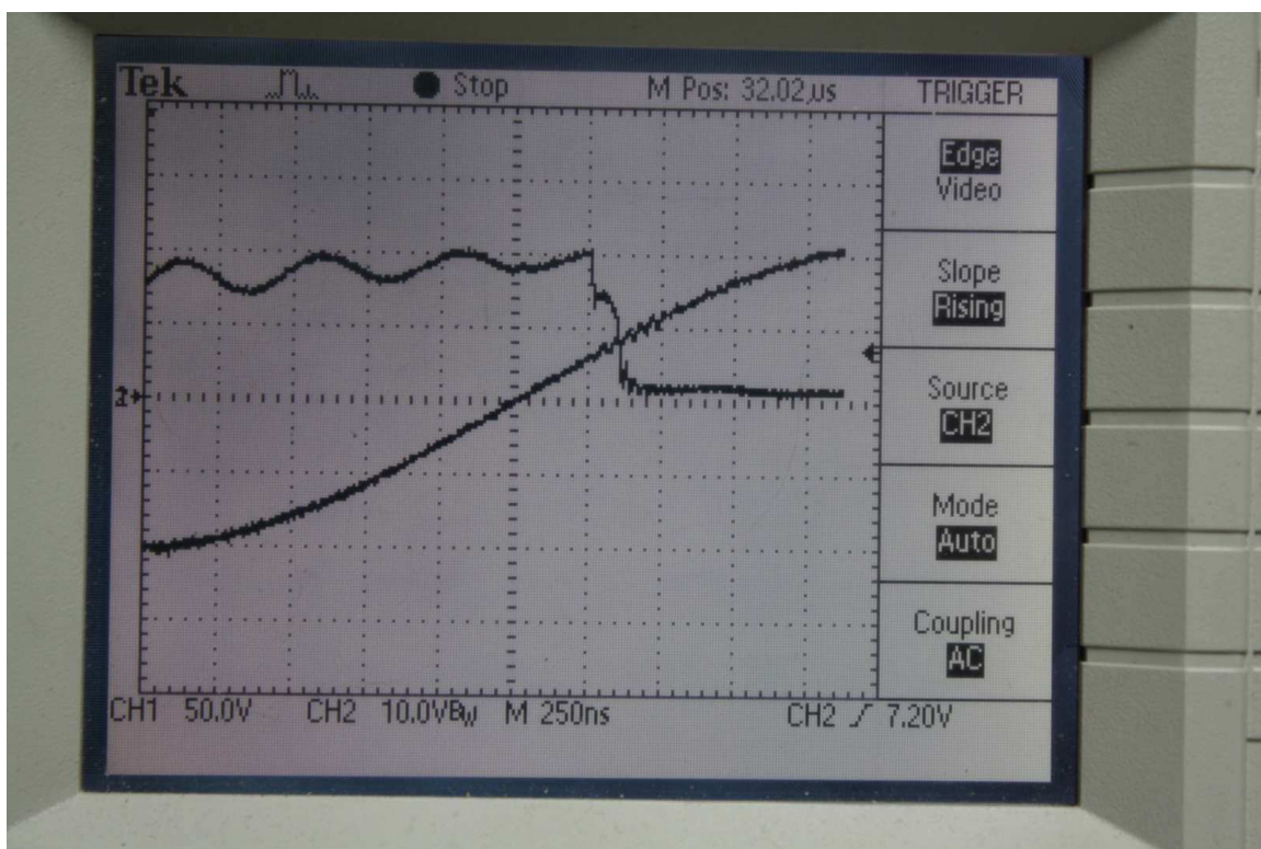
Zoom in on the IGBT turn ON
