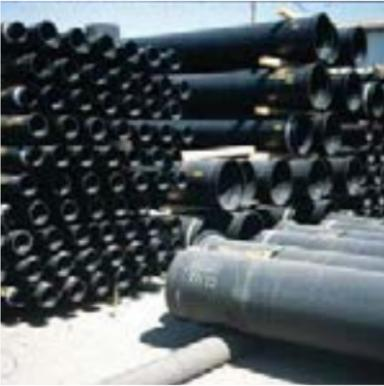
regardless of the method of transportation, it should be carefully inspected for damage that may have occurred in transit.
