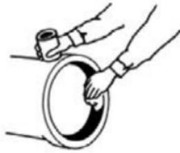
2. Apply lubricant to the exposed surface of the gasket and plain end of the pipe or fitting in accordance with the pipe manufacturer's recommendations. Do not apply lubricant to the bell socket or the surface of the gasket in contact with the bell socket. Lubricant is furnished in sterile containers and every effort should be made to keep it sterile. For underwater or very wet joint assemblies, relatively insoluble underwater joint lubricant is available and should be used.
