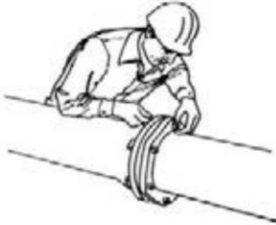
3. Push the gland toward the socket and center it around the plain end with the gland lip against the gasket. Insert bolts and hand tighten nuts. Make deflection after joint assembly but before tightening bolts.
