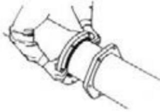
2. Insert the plain end into the socket and press the gasket firmly and evenly into the gasket recess. Keep the joint straight during assembly.
