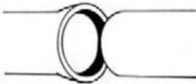
3. Be sure that the shape/dimensions of the bevel on the plain end is per the manufacturer's recommendations; square or sharp edges may damage or dislodge the gasket and cause a leak. When pipe is cut in the field, bevel the plain end with a heavy file or grinder to remove all sharp edges. Do not use a saw blade to bevel the plain end. Push the plain end into the bell socket of the mating pipe or fitting, keeping the joint straight while pushing. Make deflection after the joint is assembled.
