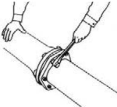
4. Tighten the bolts to the normal range of bolt torque (as indicated in the table below) while constantly maintaining approximately the same distance between the gland and the face of
